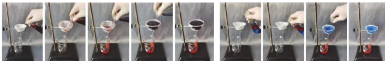
Figure 28: Applications of the PLA/CNTs filtration membrane for oil-water separation: n- hexane/saturated salt water (left) and n-hexane/water (right) [67].
