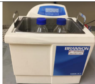
F) Sonication of the mixture using ultrasonic bath for 30 minutes at 27°C in moderate setting.
