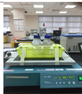
D) The MRP and MLP were mixed with ethanol using vibrator at 200rpm for 7 days.
