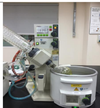
H) Evaporation of filtrate by using rotary evaporator at 40°C for 2 hours until appropriate viscosity is obtained.
